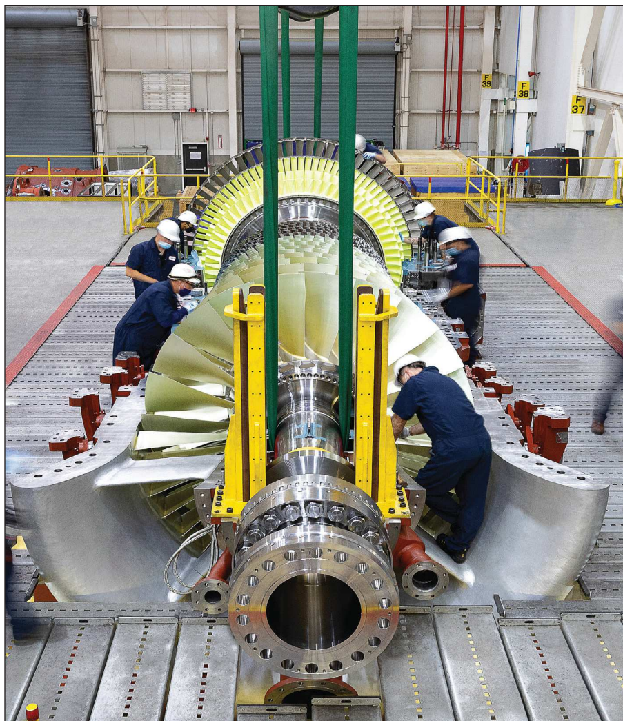
M501JAC gas turbine. Simple cycle gas turbine plant is ISO rated at 425MW base load output and 44% efficiency on natural gas fuel; single-shaft 1x1 combined cycle is rated at 630MW net plant output at over 64% efficiency.
